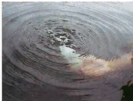
A water sample is properly obtained by lowering the bottle upside down 1-2 feet below the surface, then pointing the bottle up, allowing the bottle to fill (credit: MiCorps staff).
